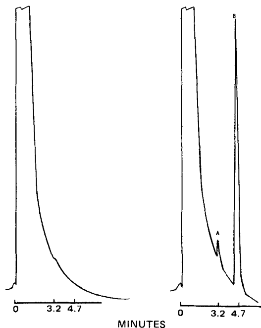
Figure 2—Chromatograms showing peaks from glycerin analysis. Key: left, control plasma; and right, plasma containing 0.09 mg of glycerin/ml and 2.0 mg of 1,6-hexanediol/ml.
